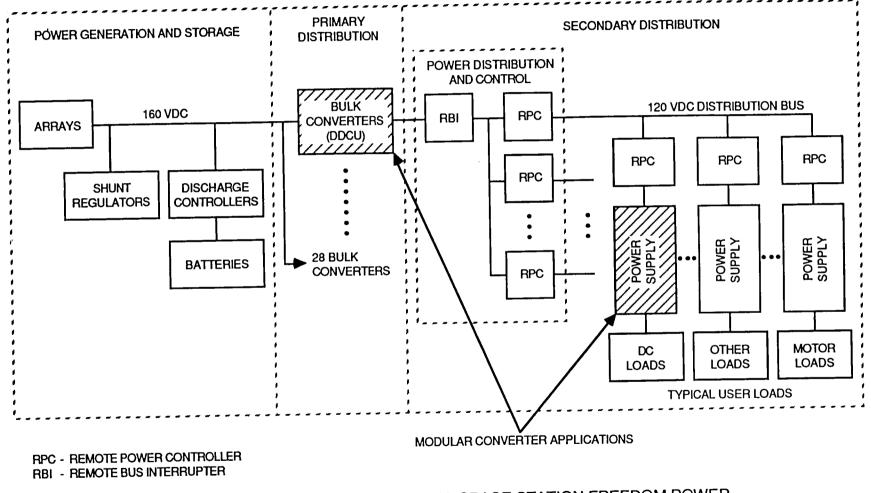
SIMPLIFIED BLOCK DIAGRAM OF TYPICAL SPACE STATION FREEDOM POWER DISTRIBUTION SYSTEM SHOWING POSSIBLE APPLICATIONS OF THE PROPOSED TECHNOLOGY
