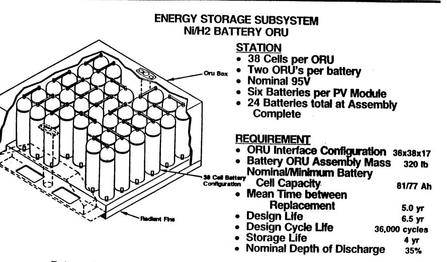
Battery ORU provides station power during solar eclipse periods
