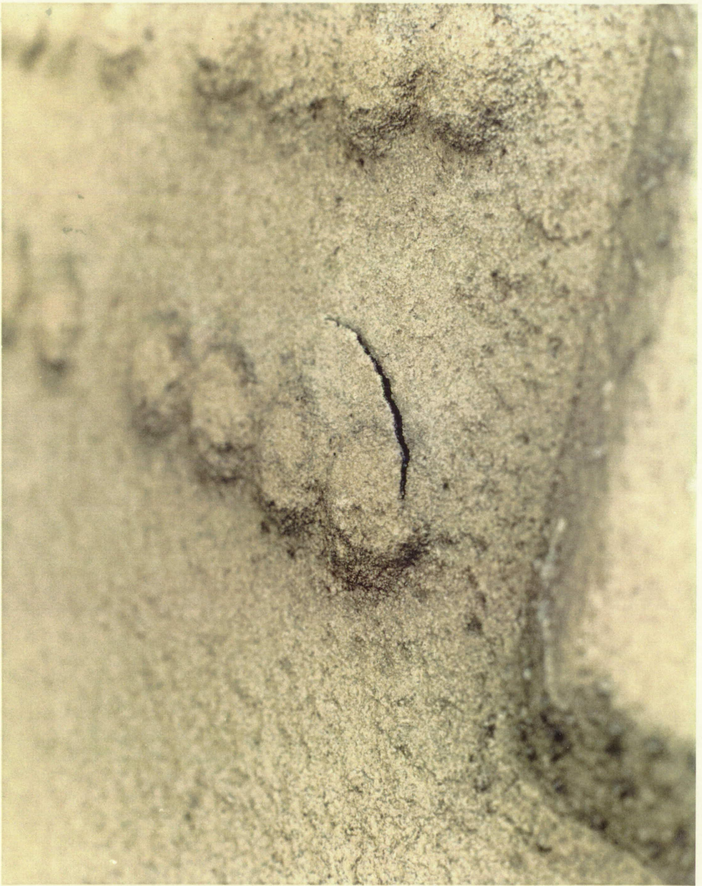
Two areas of MSA-2 were debonded on the aft skirt acreage
