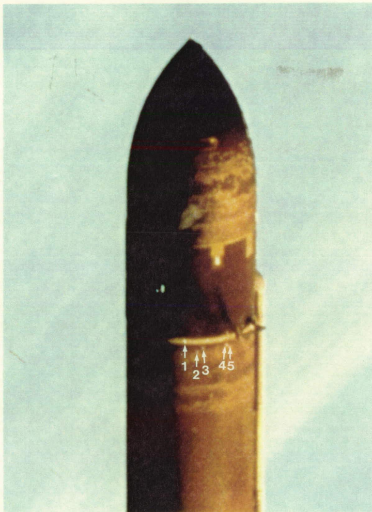
Figure 2.4.1 Divots on the External Tank
