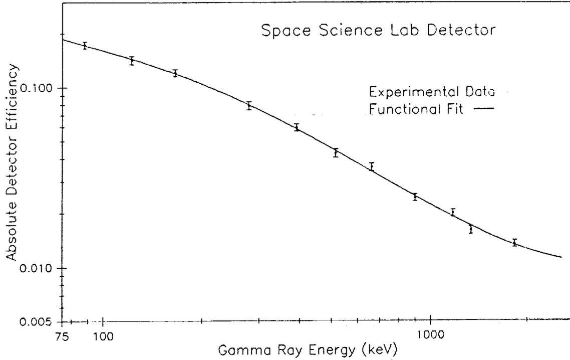
Figure 1. Efficiency Curve for SSL/MSFC Detector
