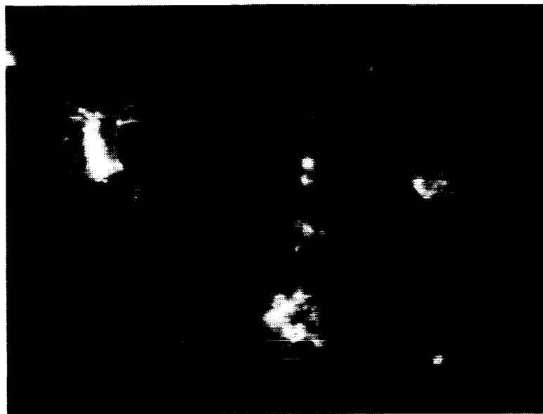
FIGURE 8: Dark field photograph showing fracture zones on a fused silica surface.
