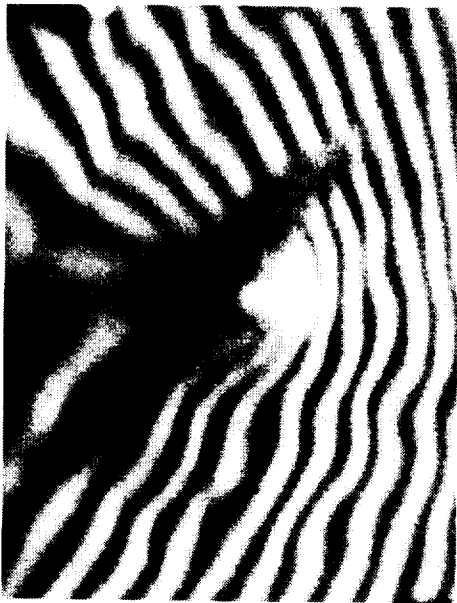
Out-of-Plane Displacement Contours
