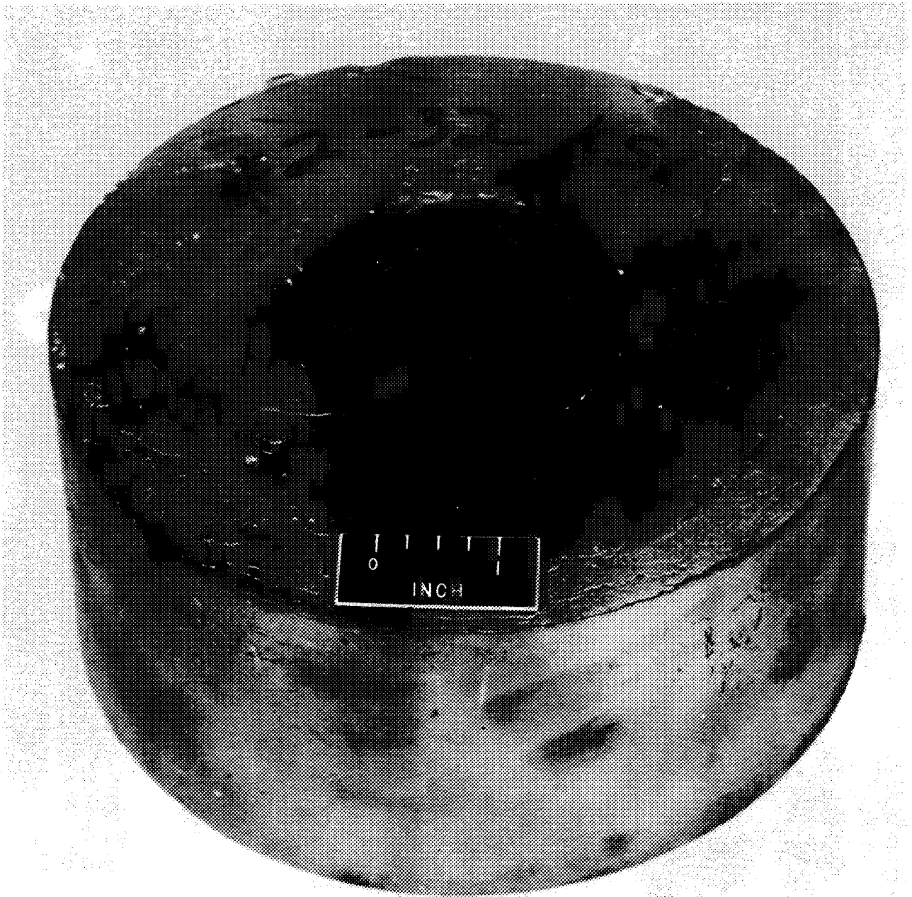
Figure 3. Typical squeeze-cast billet post processing.
