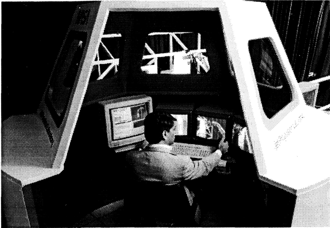
Figure 4. Remote Surface Inspection Laboratory, showing the Operator Control Station housed in a full-size cupola mockup of the Space Station.
