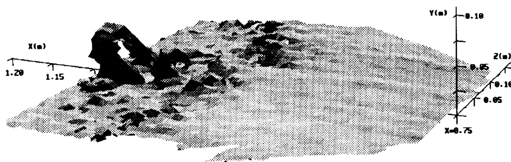
FIGURE 8. Contour surface of vorticity magnitude showing the vortex loops just downstream of the transition region.
