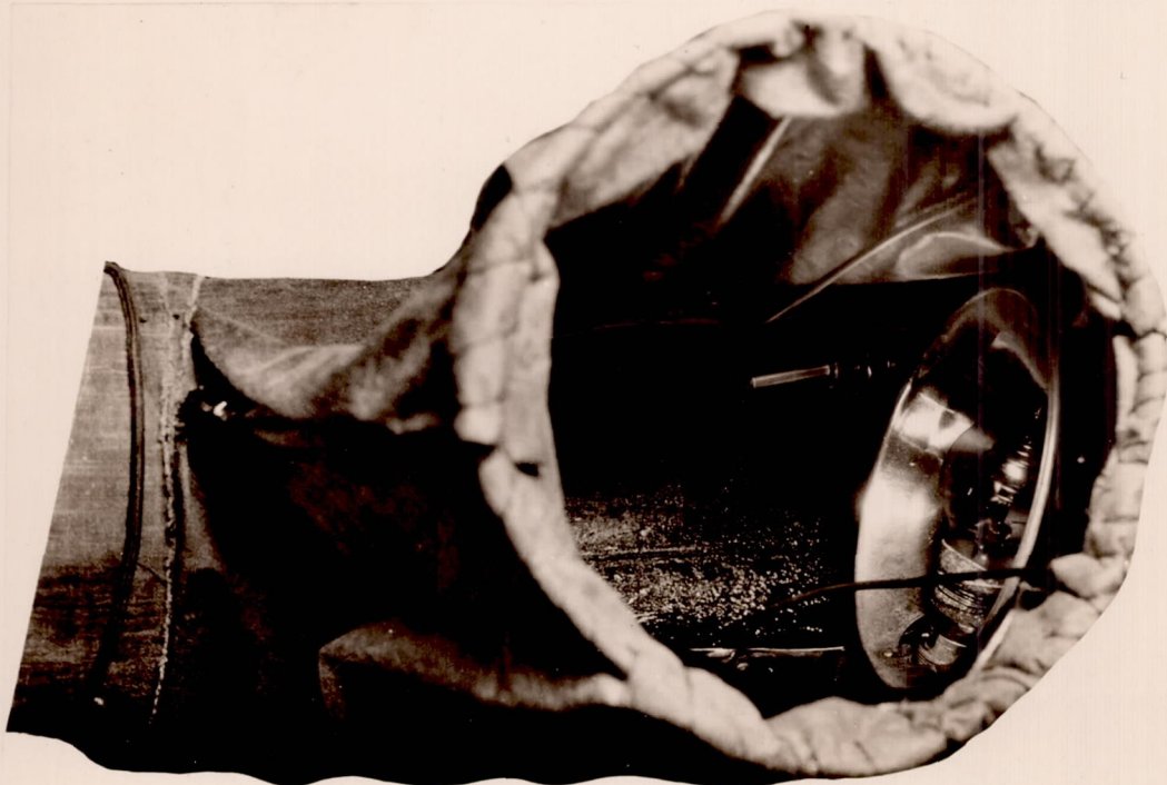
Fig.2 Position of injection valve and Neon lamp for observation of fuel sprays.
