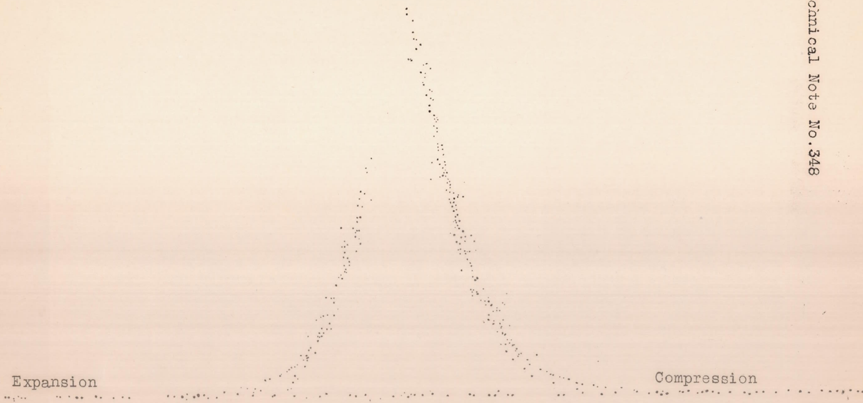
Fig.3 Reproduction of photographs of card taken with indicator as received from manufacturer. Engine motored at 1600 r.p.m. Compression ratio = 13.5.
