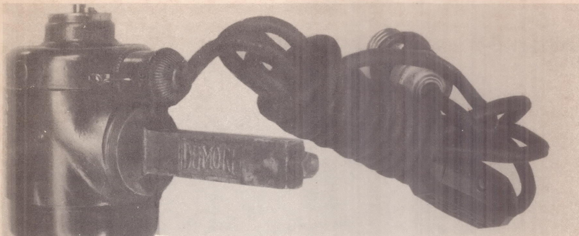
Figure 3. Motor and grinding wheel used for the "spark tests".
