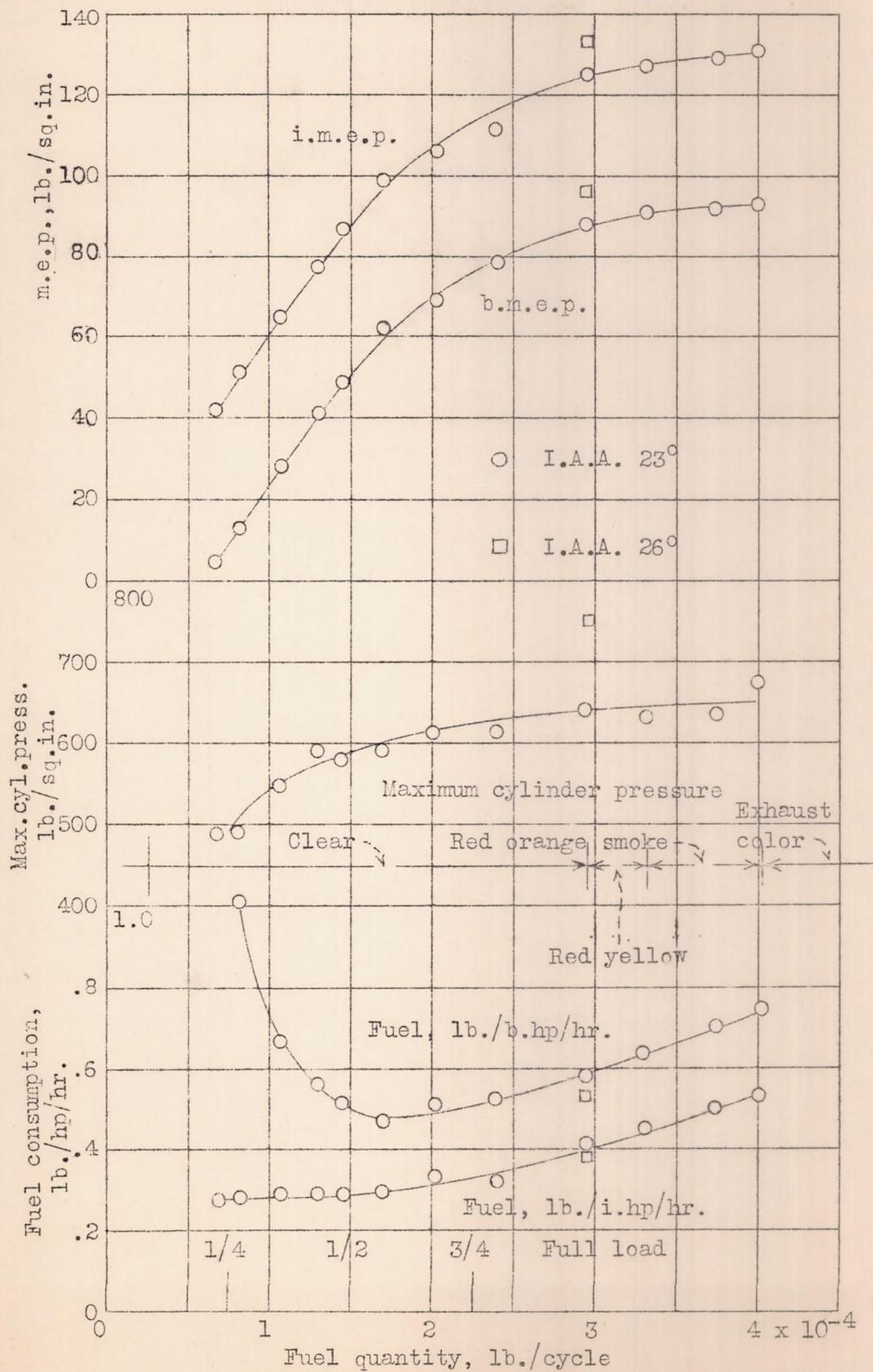
Fig. 7 Effect of load on engine performance (centrifugal spray).
