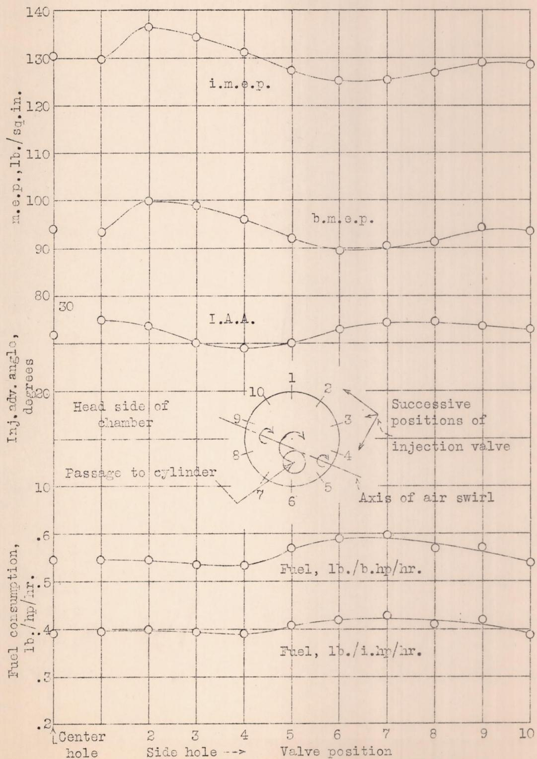
Fig. 11 Effect of injection position on engine performance (spherical chamber). 1500 r.p.m.
