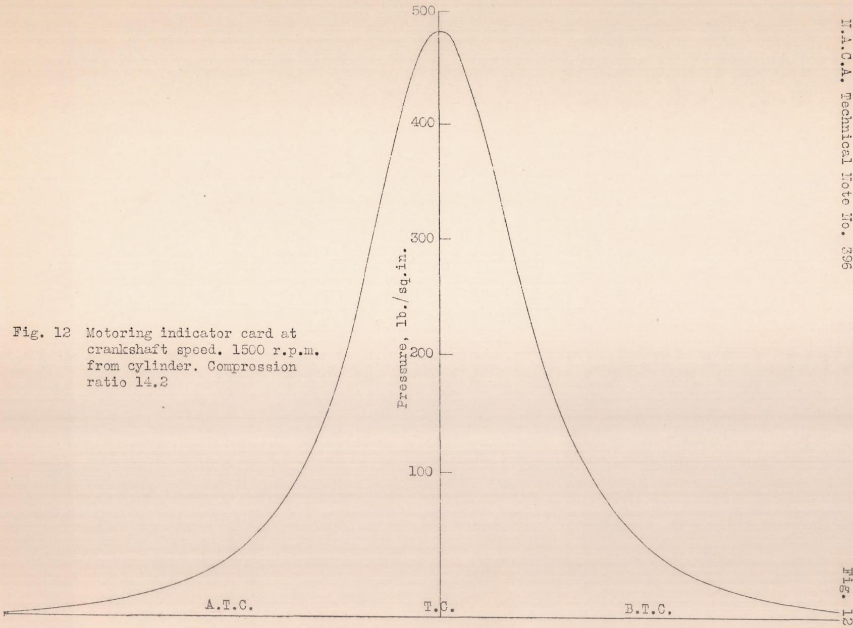
Fig. 12 Motoring indicator card at crankshaft speed. 1500 r.p.m. from cylinder. Compression ratio 14.2
