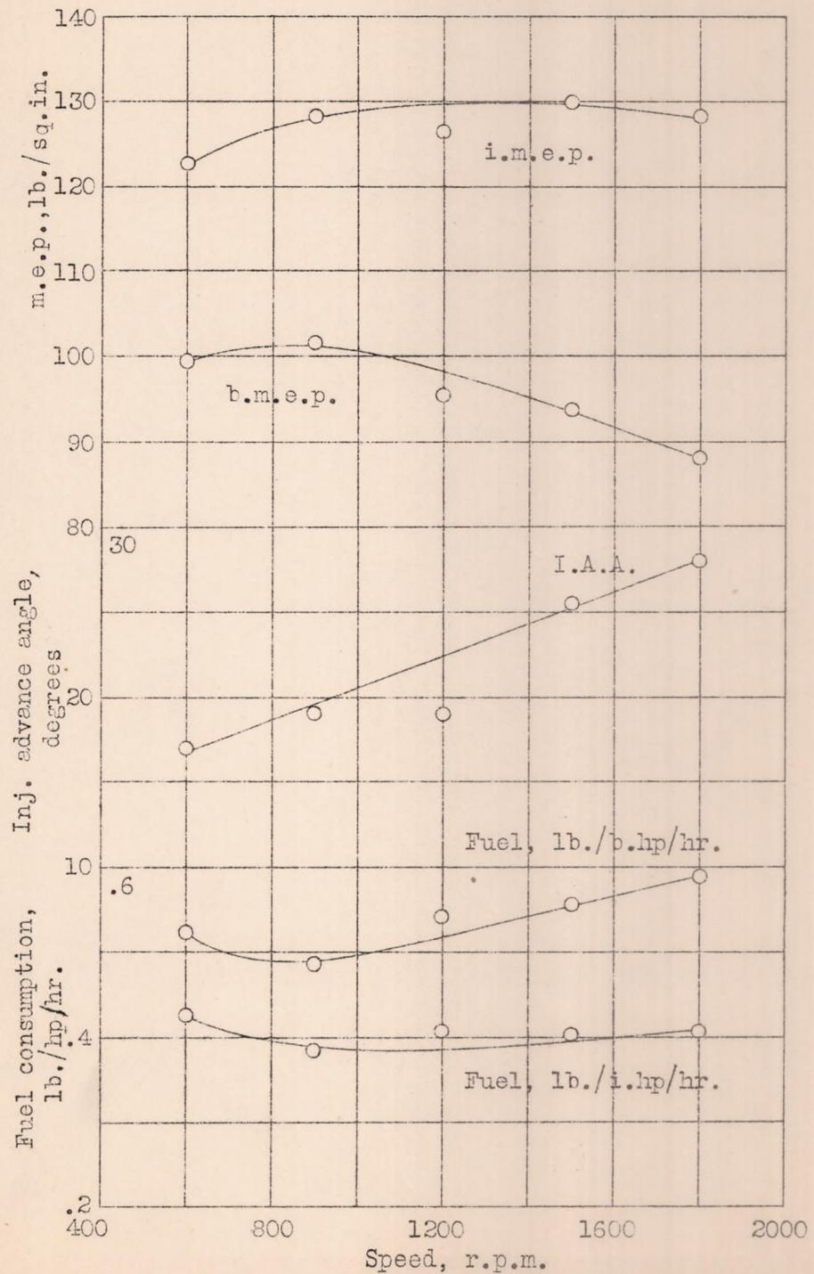
Fig. 8 Effect of speed on engine performance.
