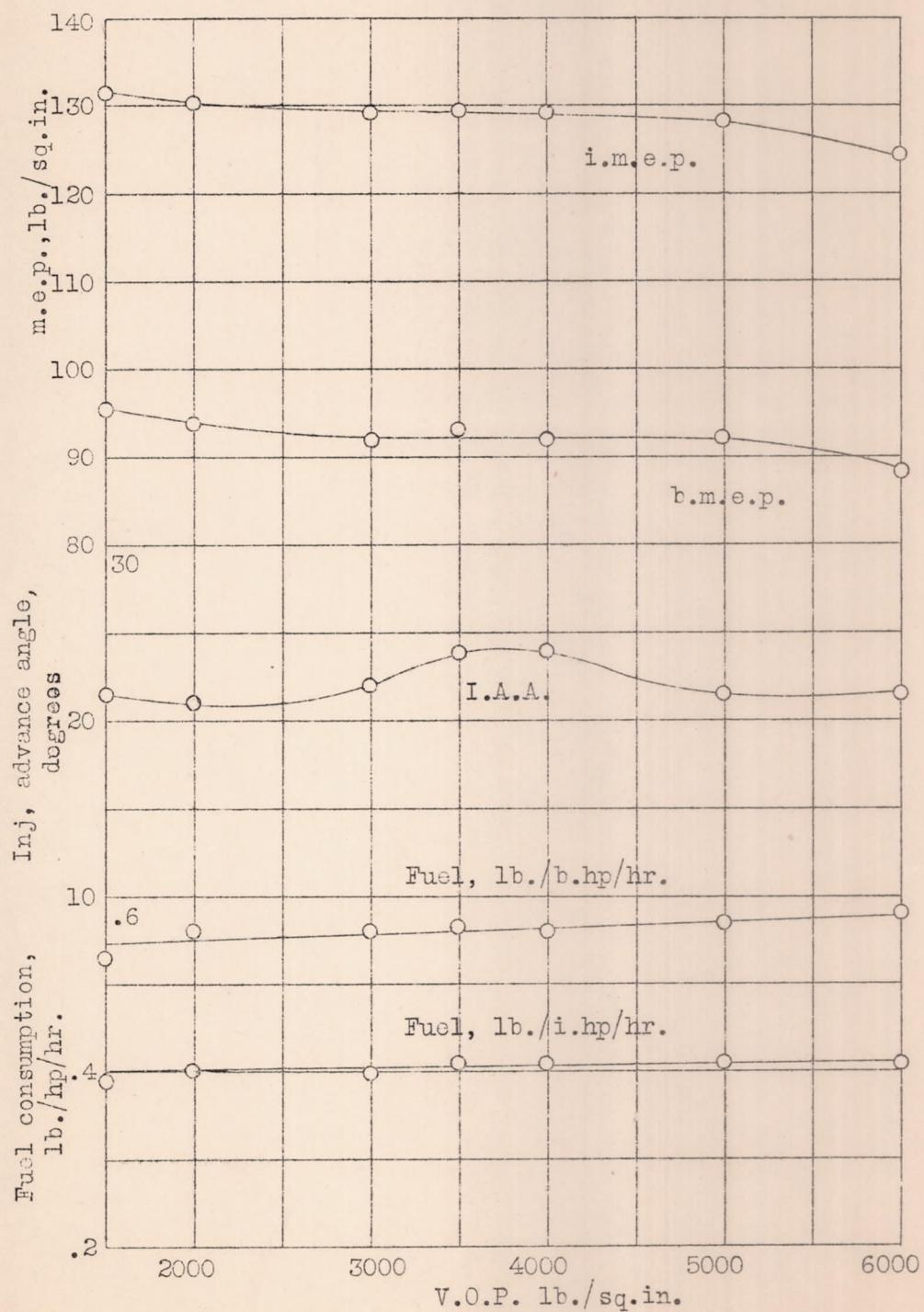
Fig. 9 Effect of valve-opening pressure on engine performance
