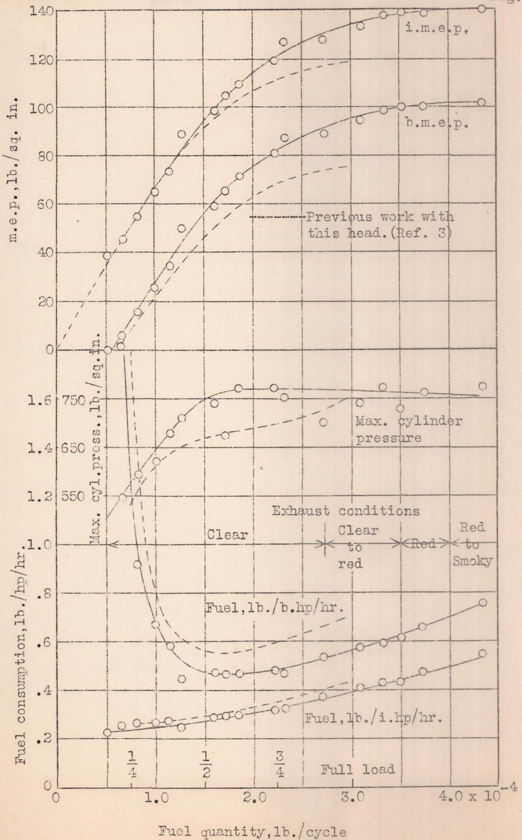
Fig.6 Effect of load on engine performance.
