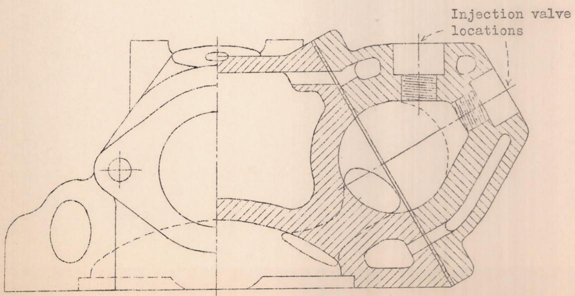
Fig. 2 N.A.C.A. cylinder-head design No. 3 showing pear-shaped and spherical (dotted) chamber forms. Passage throat diameter  $9/16$  inch.
