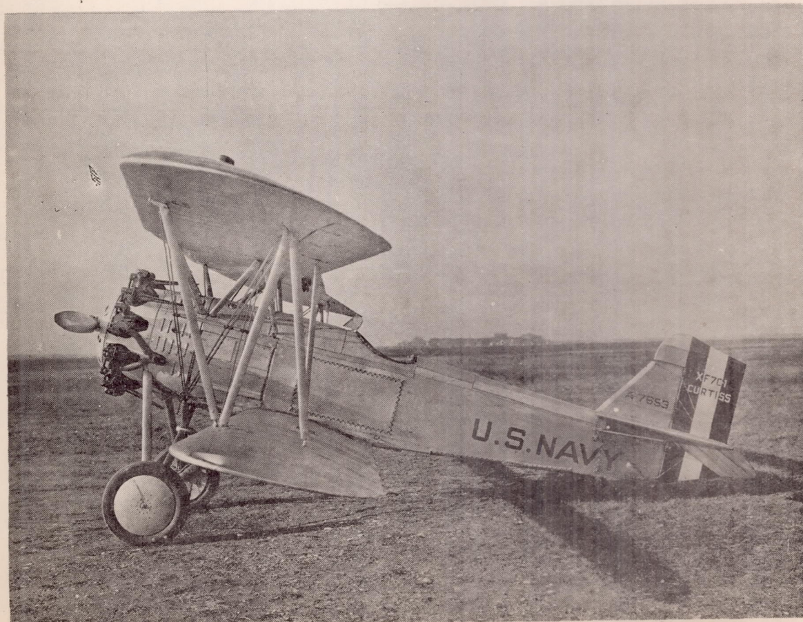
Fig.2 Side view of XF7C-1 airplane with service type fuselage and cowling.
