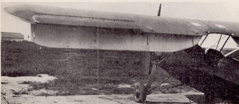
Figure 4.- Fairchild 22 airplane with Zap flaps in the down position.
