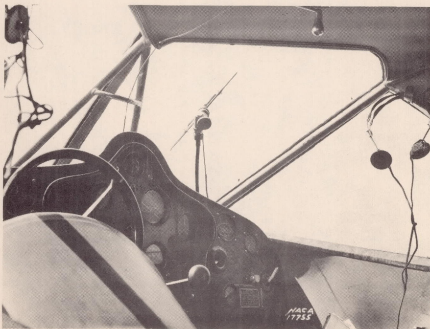
Figure 7.- An engine-driven rotating wiper blade, viewed from the interior of the airplane.
