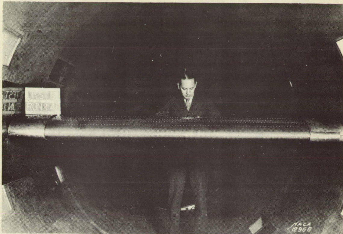
Figure 1.- 5-foot airfoil mounted in wind tunnel.
