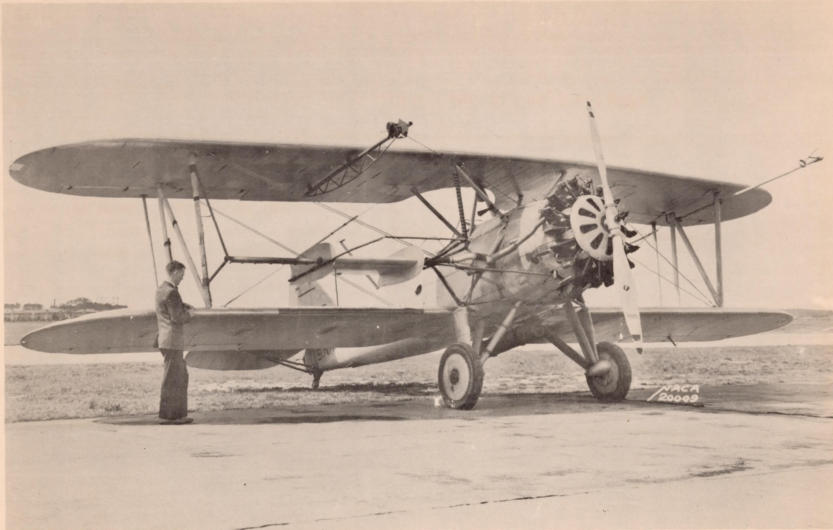
Figure 1.- General view of XBM airplane, showing wing heated by hot air, and motion-picture camera mounted above and in front of model.
