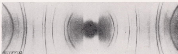
Interference lines of the K_{\alpha} radiations of Cu.
