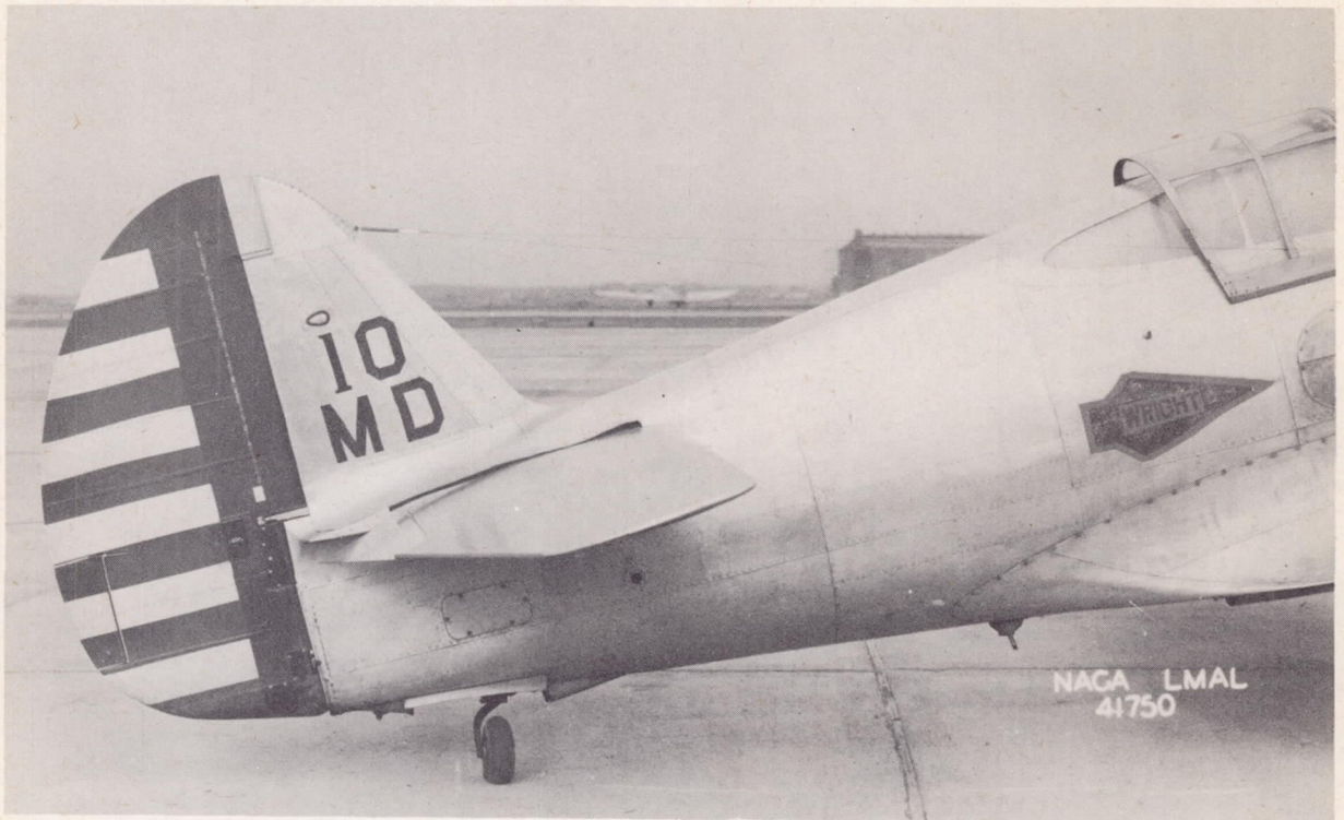
Figure 5.- All-movable horizontal tail deflected full down.
