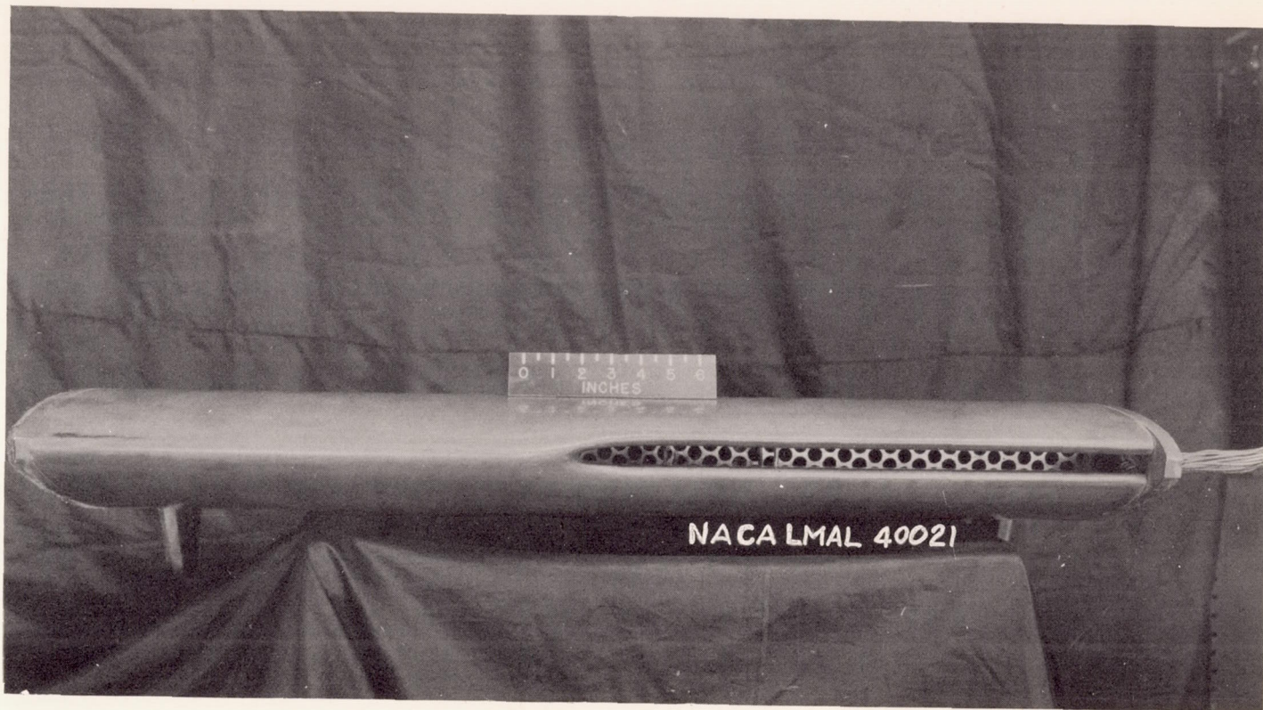
Figure 15.- Model with leading-edge air intake tested in the Langley two-dimensional low-turbulence tunnels.
