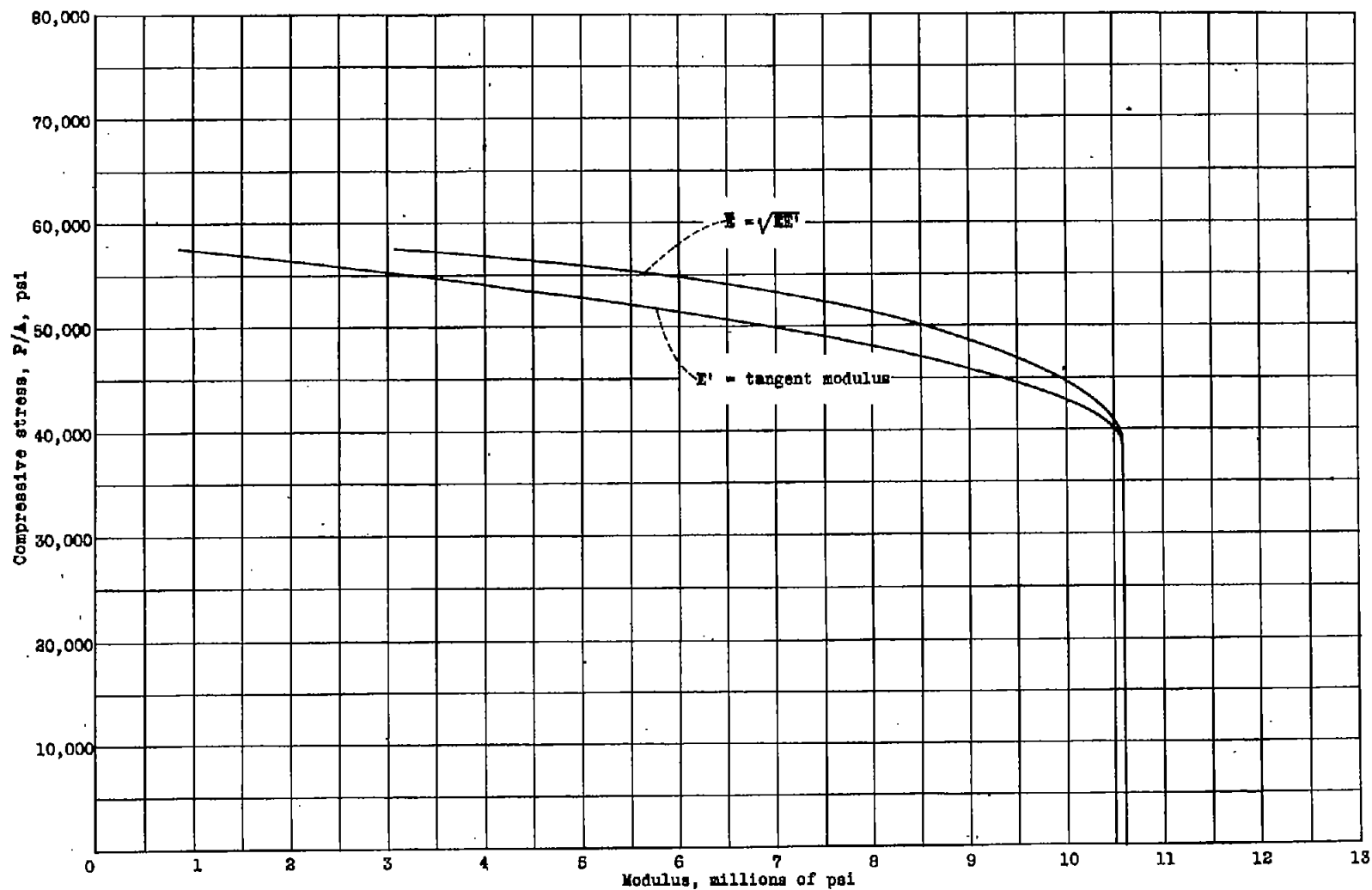
Figure 7.- Compressive stress-modulus curves. Relations derived from compressive stress-strain curve for 2-1/2 x 2-1/2 x 1/4-inch extruded 14S-T angle. Compressive specimen=5/8-inch wide x full thickness. Strains measured with Huggenberger tensometer.
