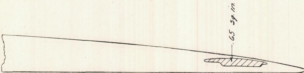
Figure 5.- Sketch of air-ported propeller-tip discharge nozzle.
