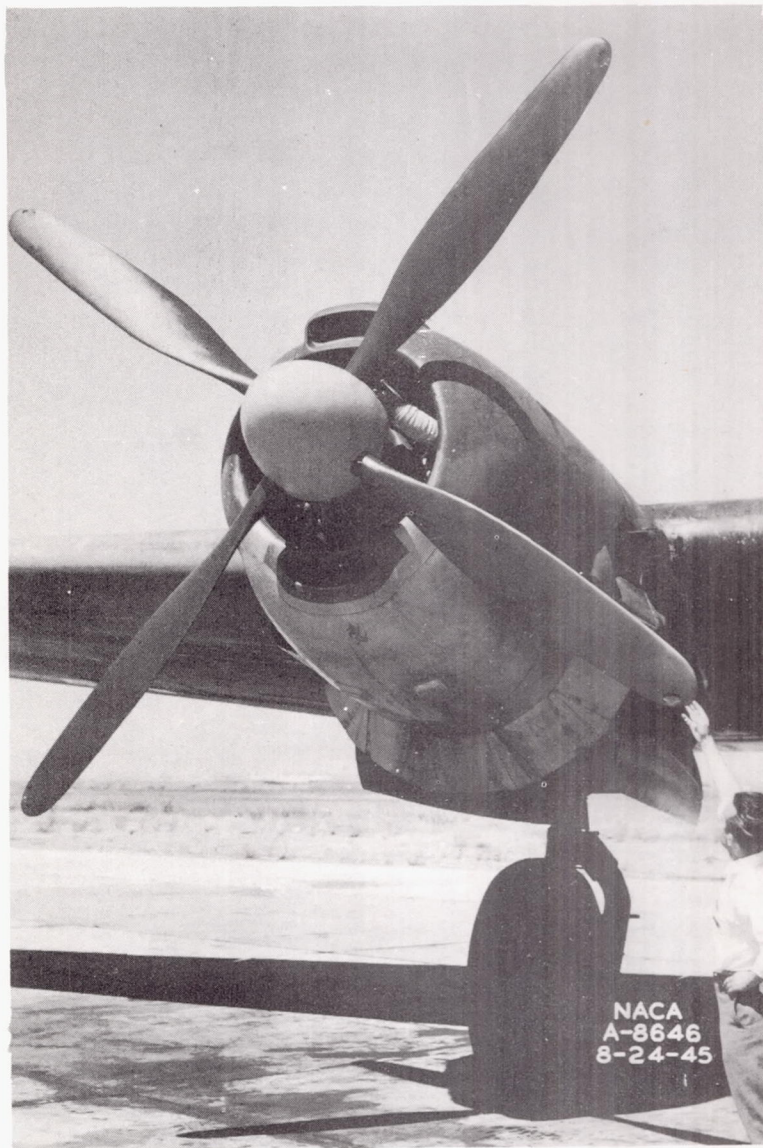
Figure 1.- Air-heated propeller installed on the right engine of the test airplane.
