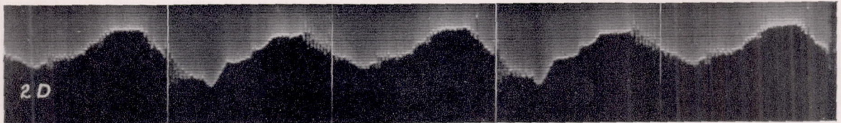
Figure 19.—Effect of manifold pressure on piston-ring friction.
