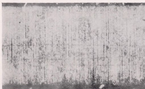
Figure 31.—Photomicrographs of surface replicas of cast-iron rings used in runs D, E, and F. (25×).
