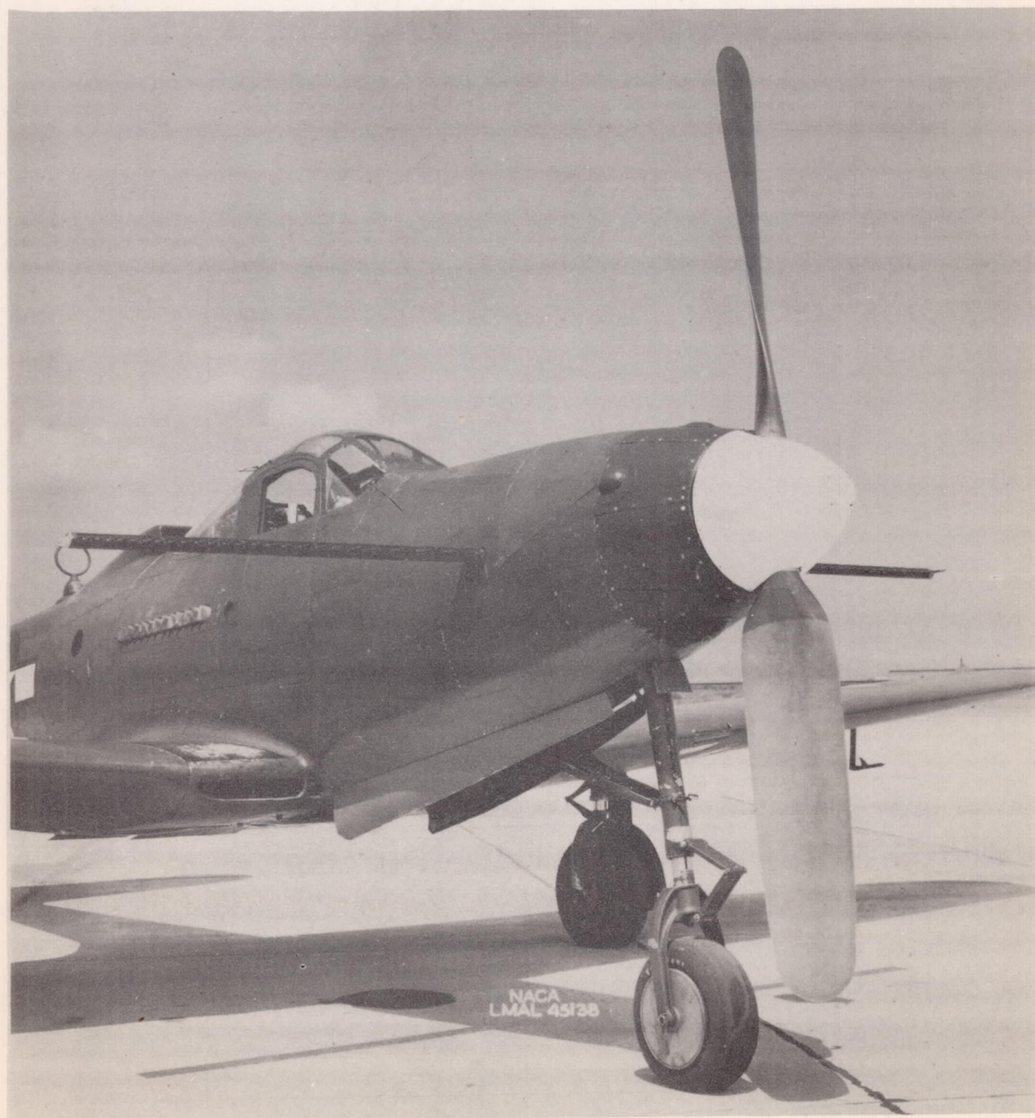
Figure 1.- General view of propeller mounted on airplane showing rapid transition from thin airfoil sections to round blade roots.
