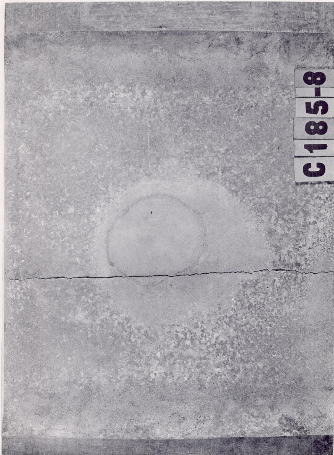
Figure 8.- Fatigue failure of welded specimen at edge of weld.
