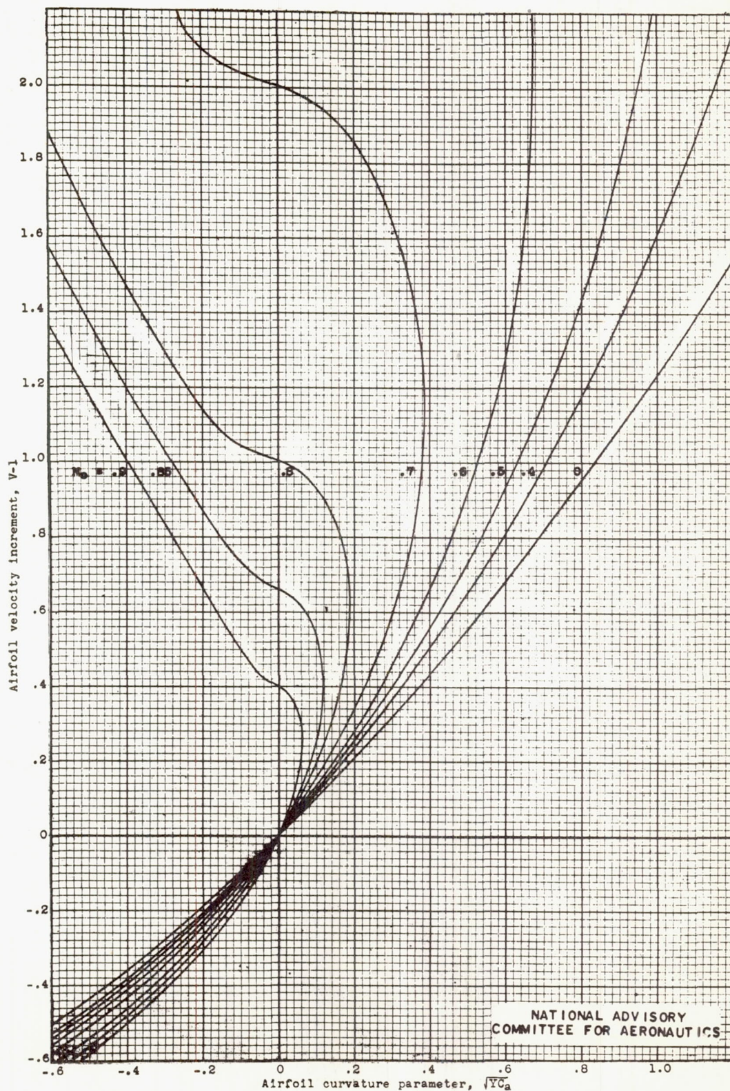
Figure 2.- Positive velocity increment on airfoil as a function of airfoil ordinate Y and airfoil curvature C_a for various values of free-stream Mach number M_0 . Values computed from equation (10) and tabulated in table I. \eta = 1.0 .
