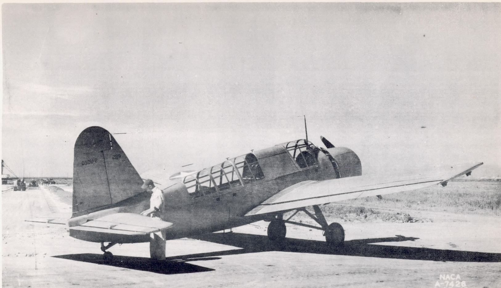
Figure 2.- The double-hinged horizontal-tail surface installed on the test airplane.
