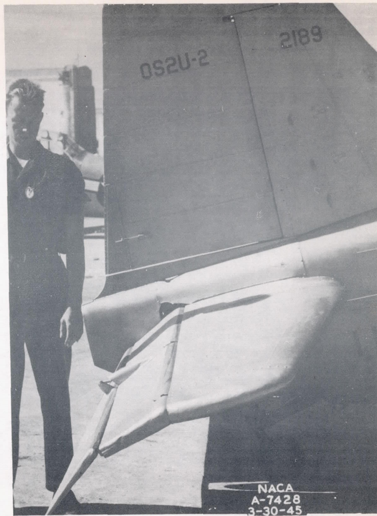
(a) Trimmer full down, elevator full up. (b) Trimmer full down, elevator full down. Figure 3.- Side view of the double-hinged horizontal-tail surface, trimmer and elevator deflected.
