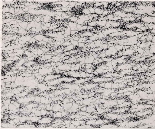
(a) Specimen F2Z; 1124 hours at 1200° F and 35,000 psi.
