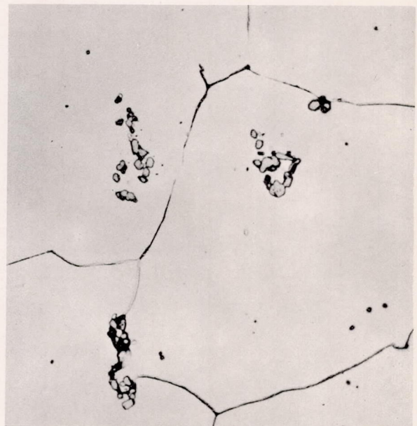
(a) Solution-treated - heated at 2100^{\circ}\text{F} 4 hours and water-quenched.
