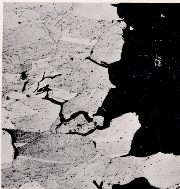
(a) Specimen 11Y; 1537 hours at 1200° F under 50,000 psi.
