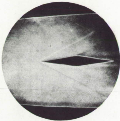
(a) Schlieren, p_0 = 180 millimeters. Arcs off.
