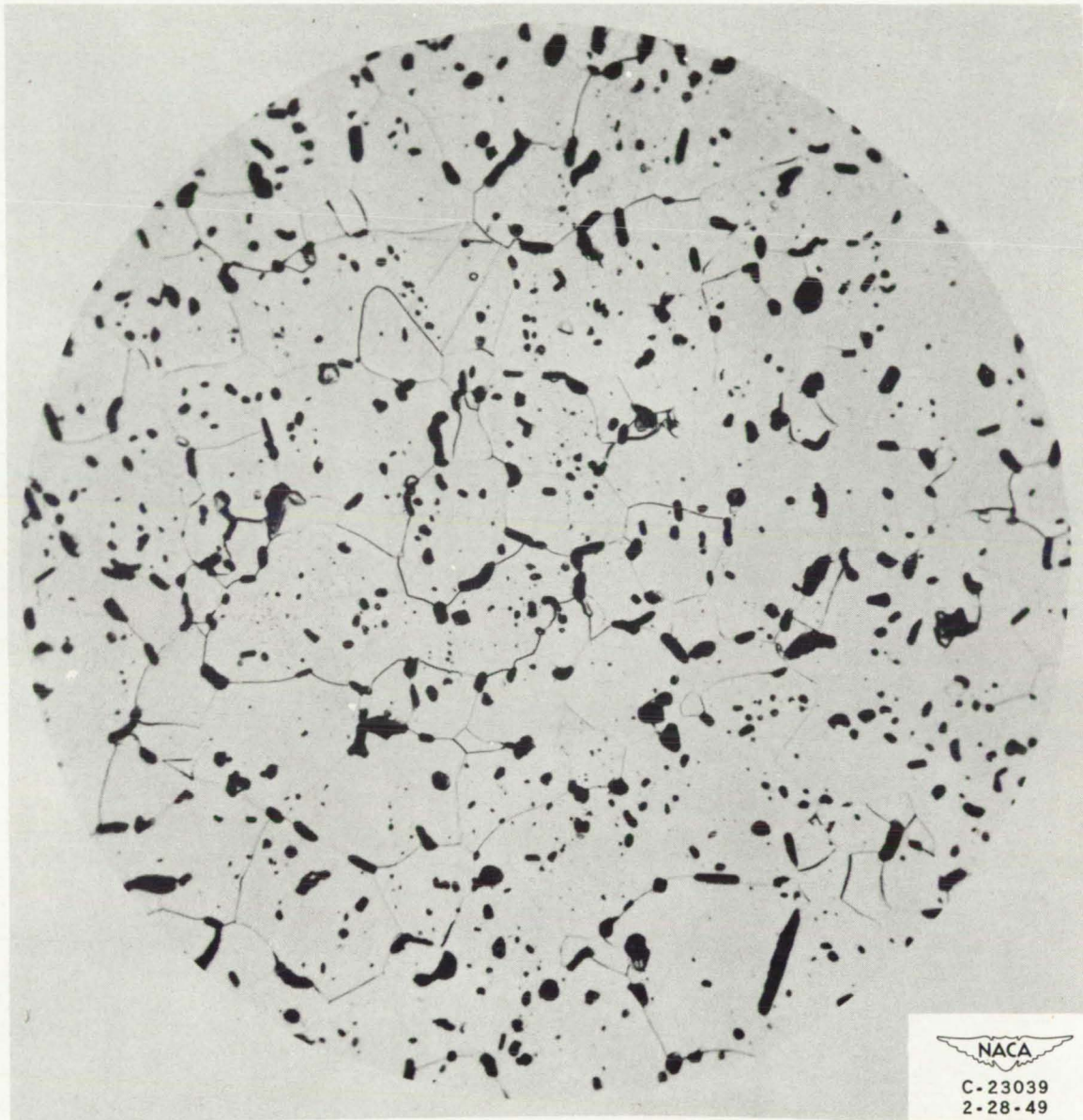
Figure 2. - Titanium-carbide specimen etched with potassium hydroxide plus potassium ferricyanide x 1500.
