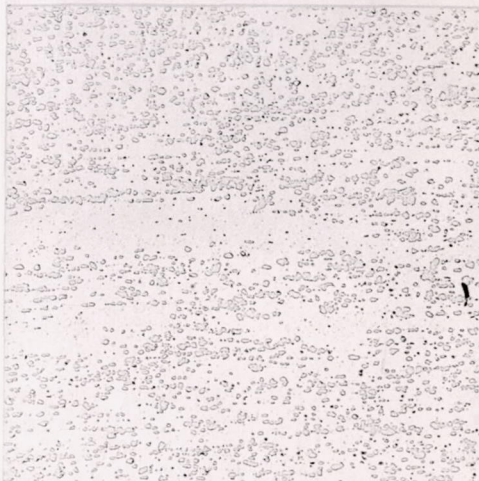
(b) Heat A2983; center of a longitudinal section from a 3/4-inch-diameter extrusion; reduction 16:1, 93.75 percent.
