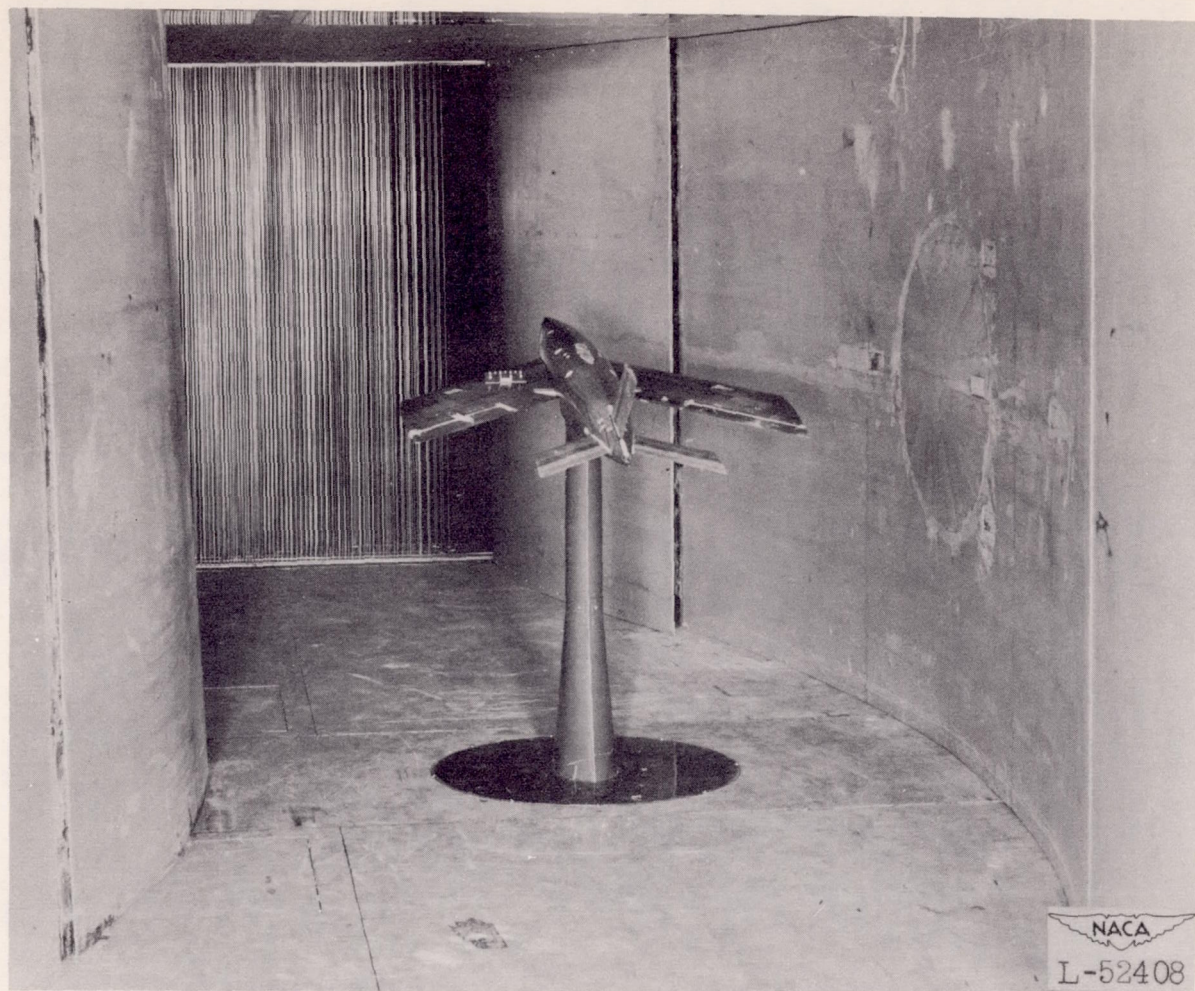
Figure 2.- Model mounted in curved-flow test section of the Langley stability tunnel.
