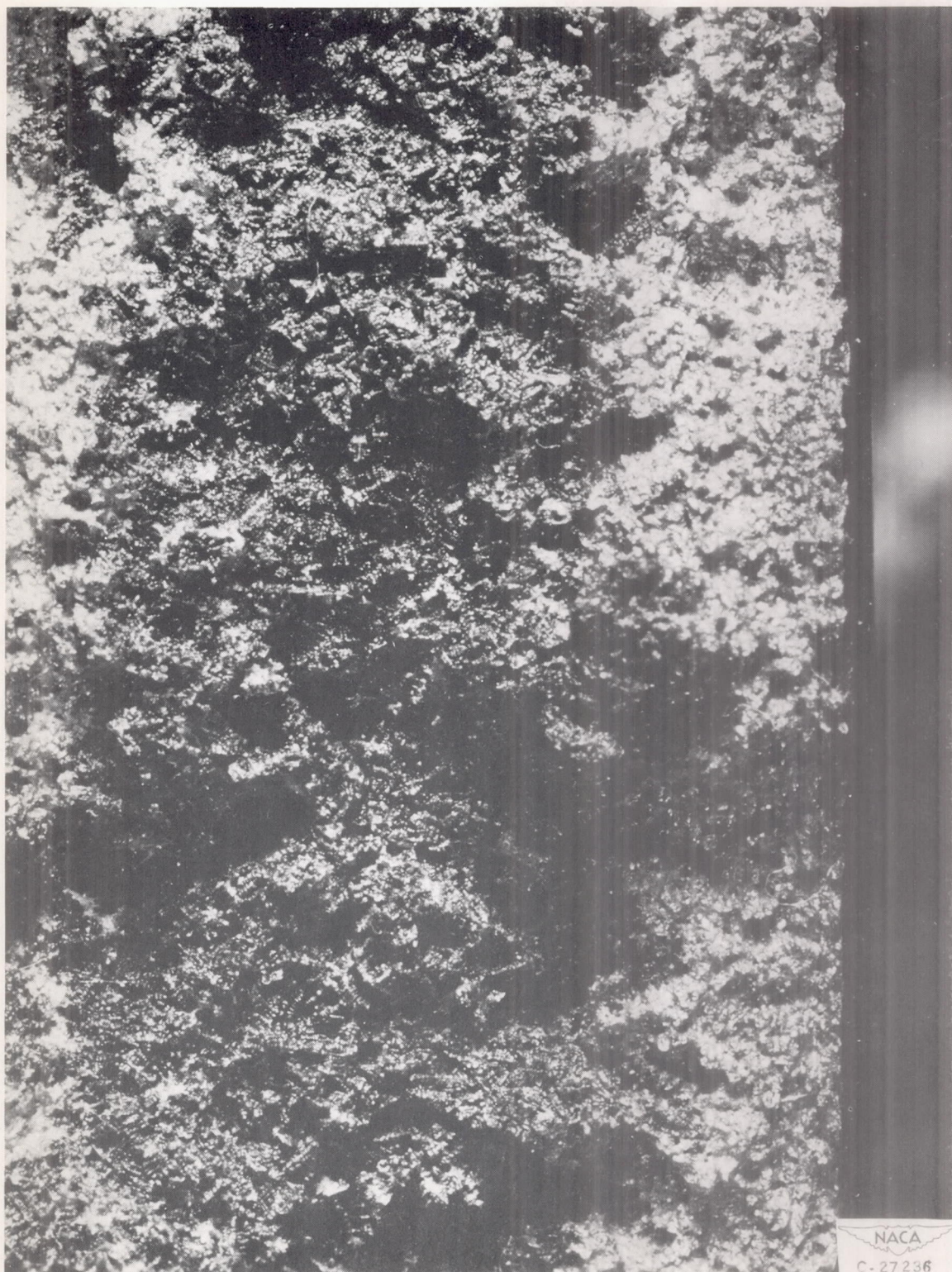
(c) Enlarged view of shrinkage area shown in figure 10(b); X11.
