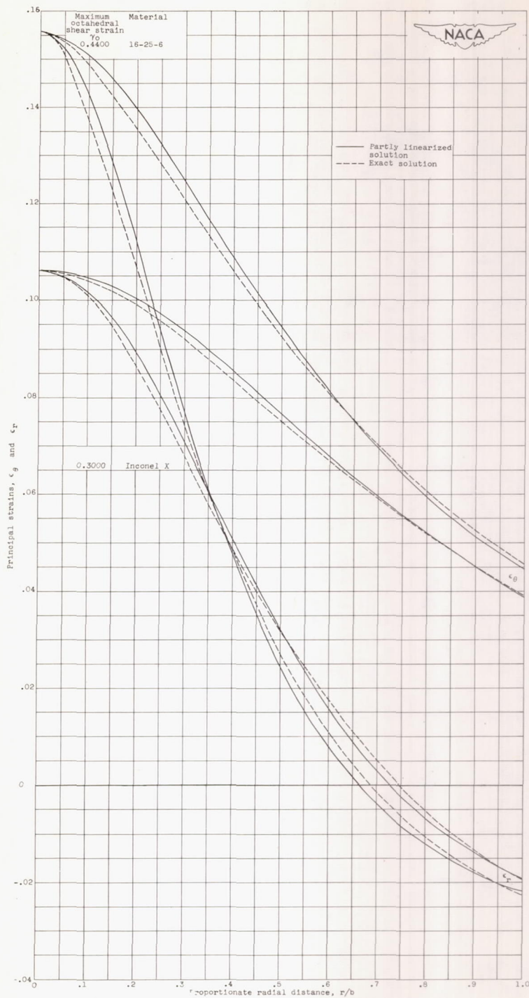
(a) Variation of principal strains with proportionate radial distance. Figure 6. - Comparison of principal strains and stresses obtained by partly linearized solution and exact solution.
