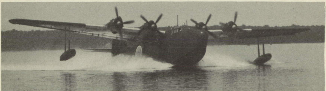
Figure 11.- Spray pattern when taxiing at 20 knots. Note action of inboard spray strips. \Delta_O = 49,900 pounds.
