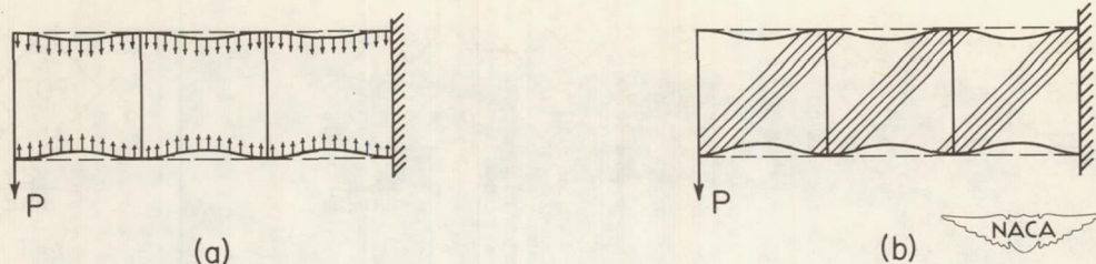
Figure 5.- Secondary actions in diagonal-tension beams .
