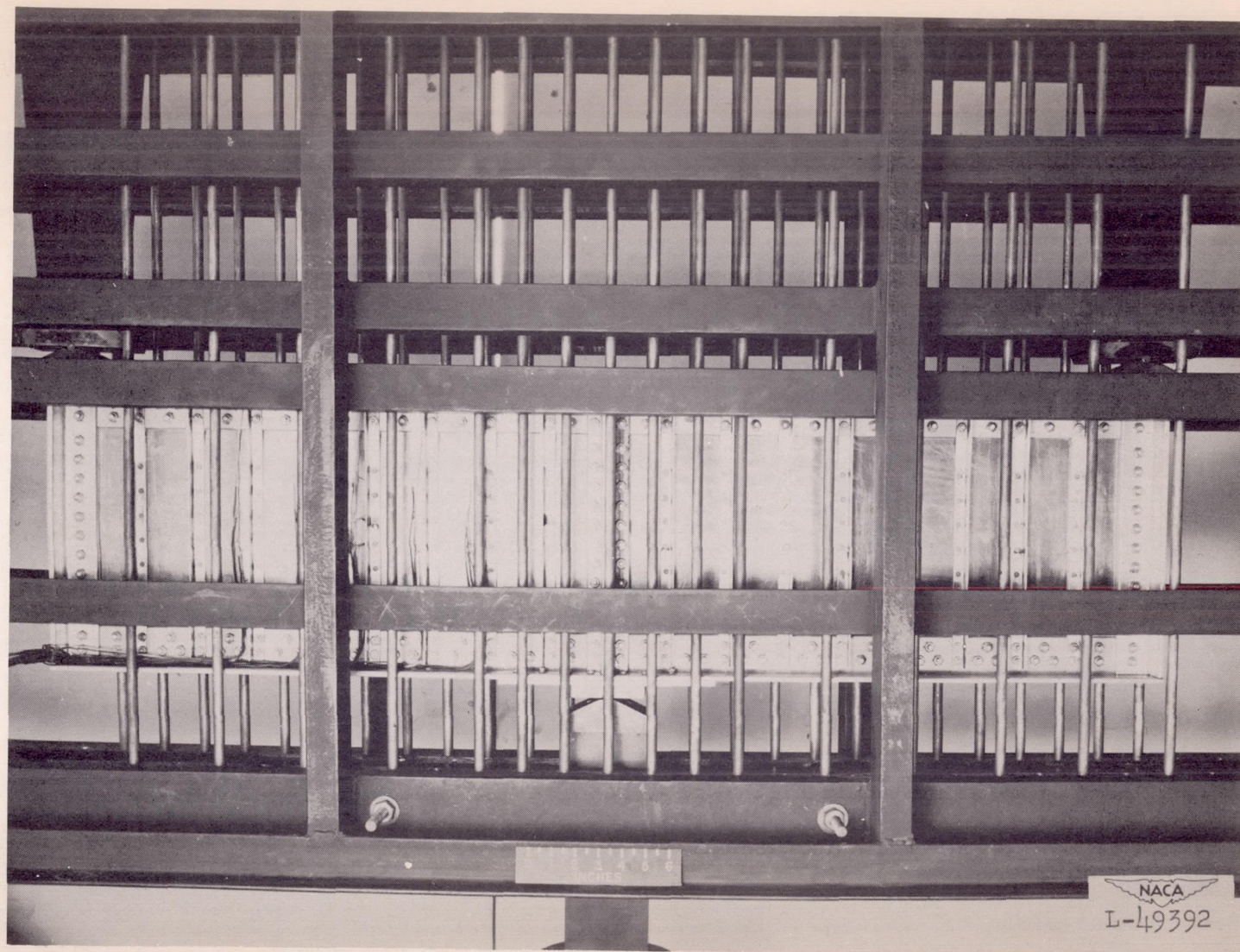
Figure 2.- Test setup for small, heavily loaded beam.
