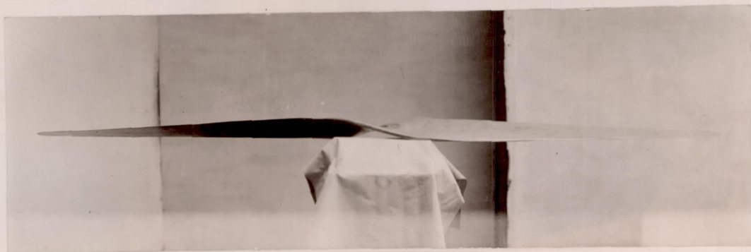
Fig. 10 - Reed 8'7" duralumin propeller \frac{5}{8} " thick at hub section; \frac{1}{8} " at tip section; made of a single piece of sheet metal \frac{5}{8} " thick. Pitch 5 feet.
