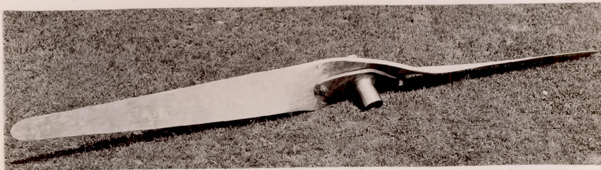
Fig. 11 - Reed duralumin propeller with twisted flange hub.
