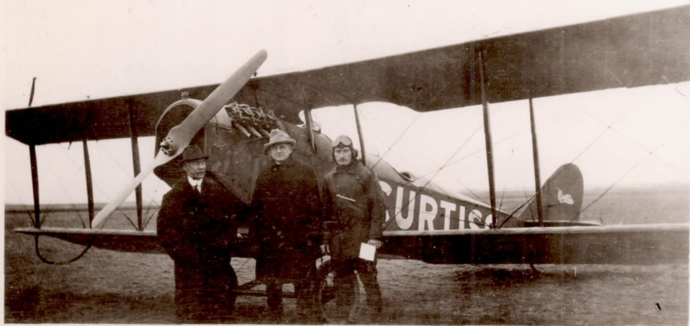
Fig. 1- Reed duralumin propeller D-4 mounted on a Curtiss JN with OX5 engine.
