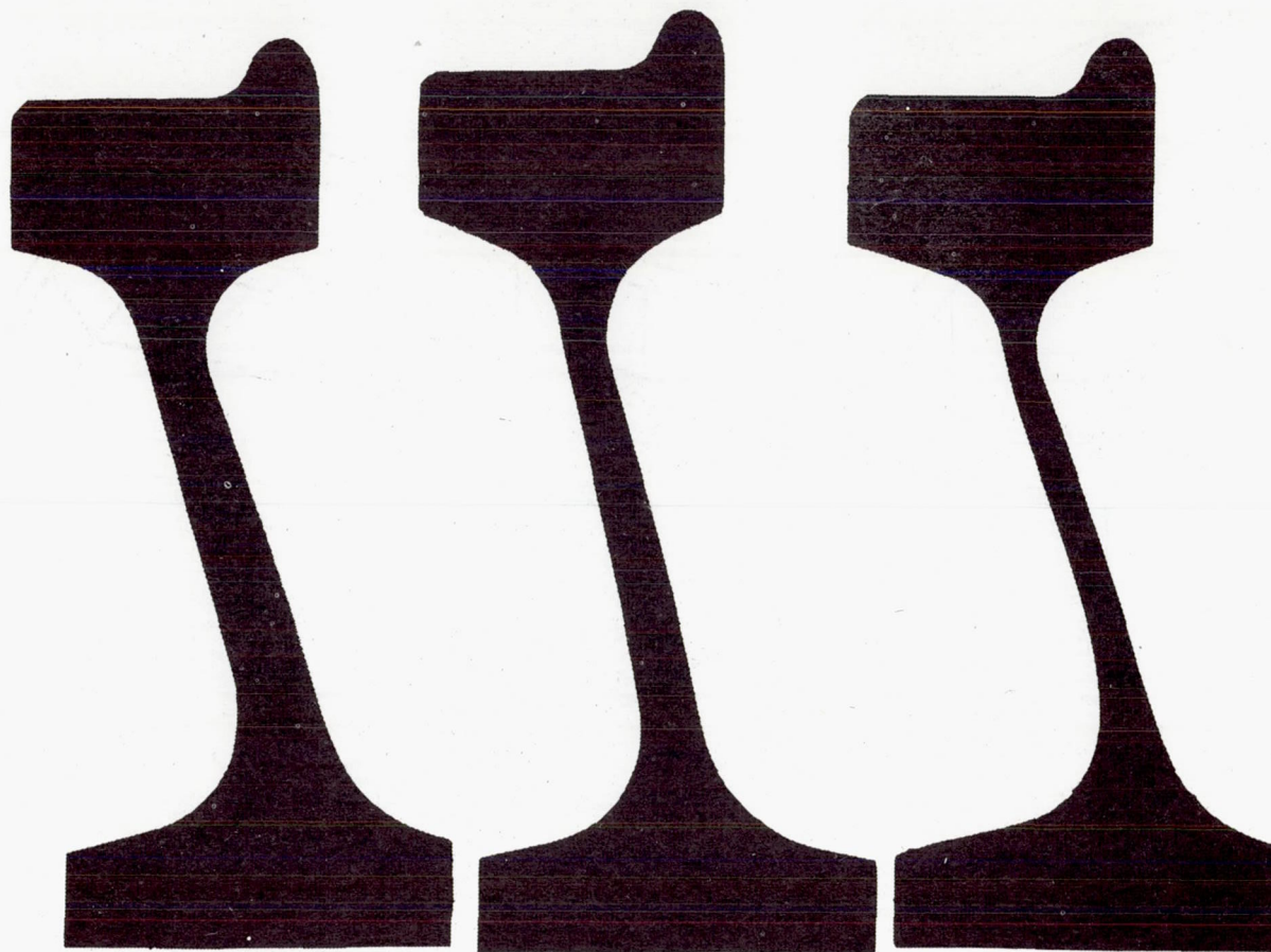
Figure 40. - Cross-sections of thick, intermediate, and thin plate wheels.
