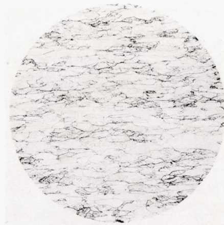
(c) Swaged 50 percent from 0.177-inch diameter recrystallized rod.
