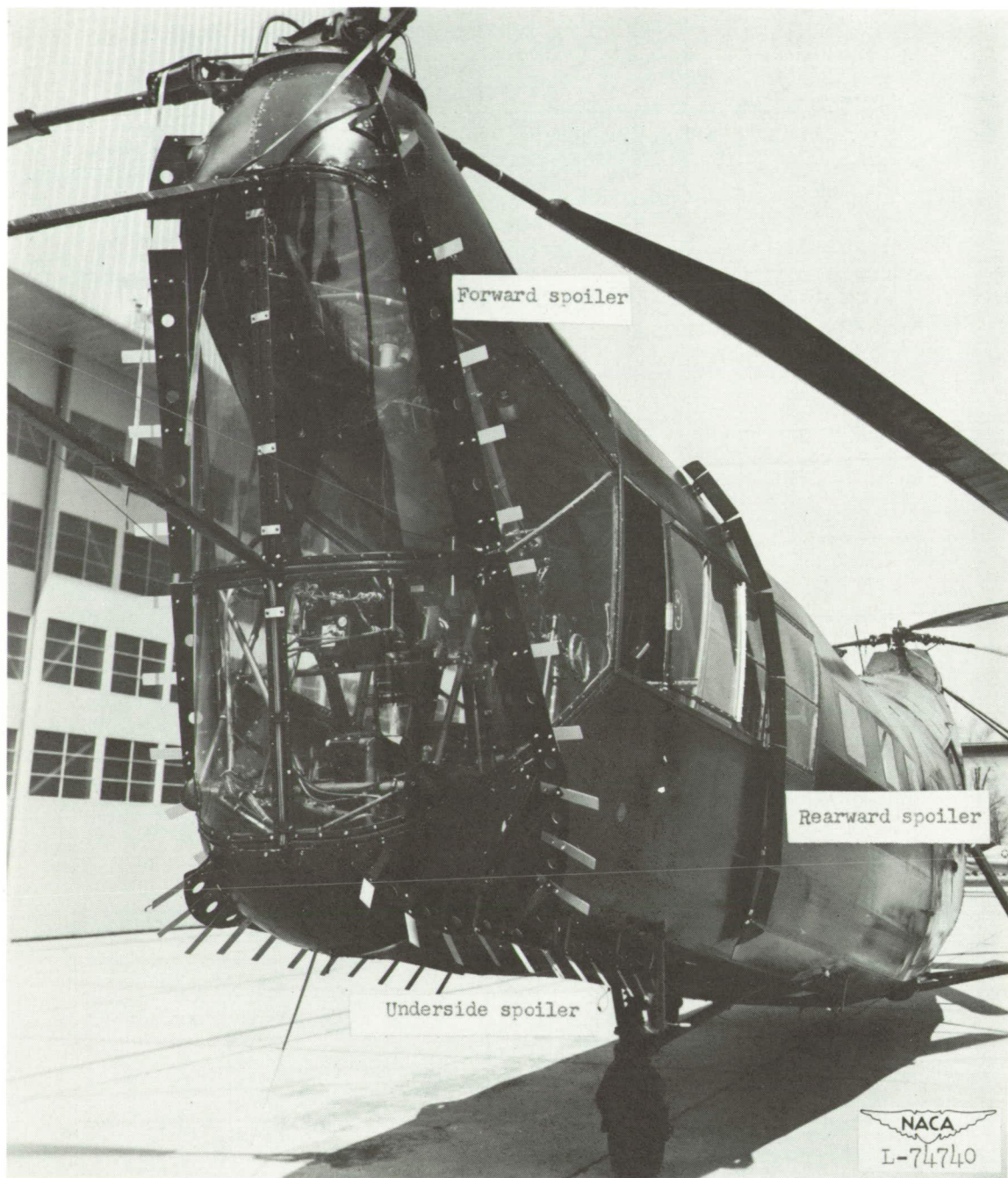
Figure 4.- Spoiler installation on test helicopter.
