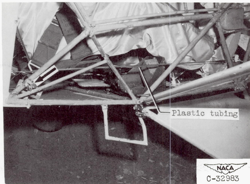
(k) Ground braid, and plastic tubing over control cable, to eliminate extraneous noise.
