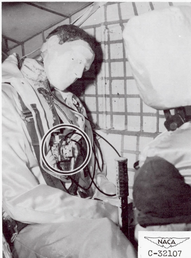
(e) Accelerometers installed on chest of rear dummy.
