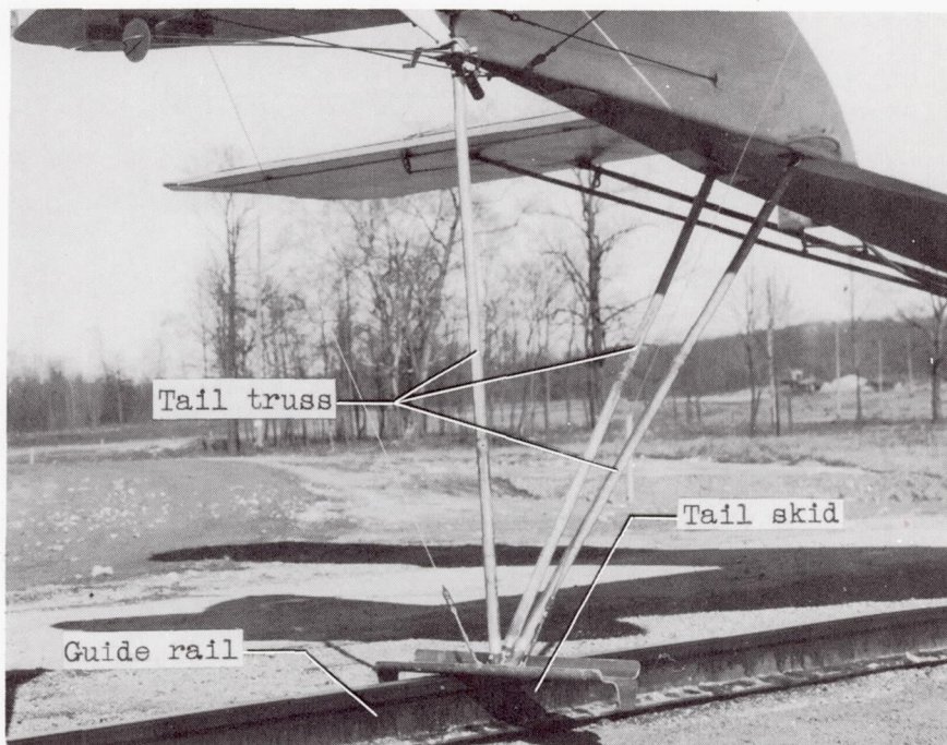
(e) Extended tail-truss support for holding airplane in flight attitude.
