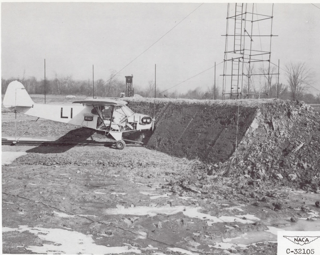
(a) Photograph of two-seat tandem airplane used in investigation, showing relation of airplane engine and left wing to front edge of earthen crash barrier.
