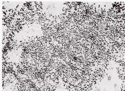
(a) As-cast condition; etchant, 10 percent NaCN in water, electrolytic.
