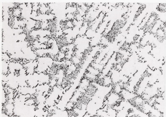
(b) Heat-treated at 2250° F and quenched (heat treatment A); etchant, 10 percent NaCN in water, electrolytic.
