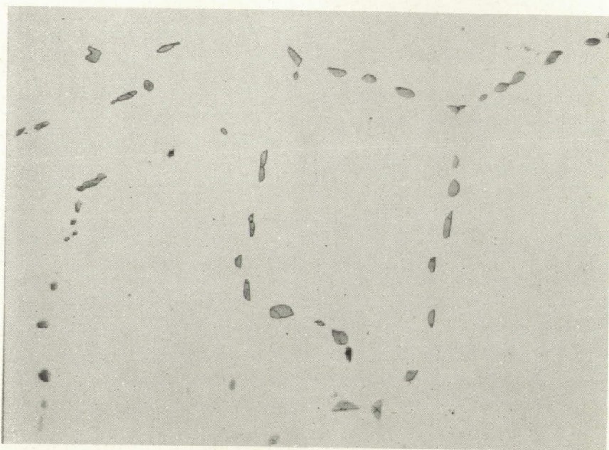
Figure 18.- Alloy 471 containing 28.83 percent chromium, 64.8 percent cobalt, and 6.37 percent molybdenum. Etched and stained according to procedure 3; small particles of stained sigma phase outlining grains of unstained alpha phase; X500.
