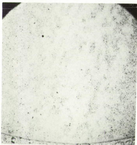
Figure 38.- Photomicrograph and autoradiograph of carbon-14 in steel. Sample coated with evaporated silver layer under autoradiograph. Collodion type AW. 1.3-hour exposure.
