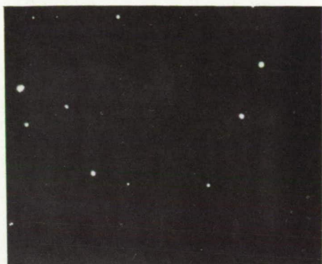
(a) Collodion and silver nitrate at 2° C. No warmup before development. 250X.
