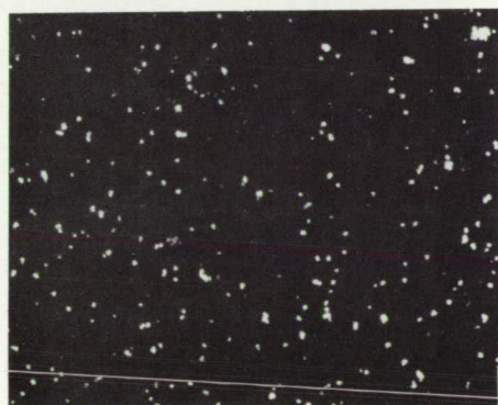
Figure 21.- Fog level produced during 1-hour autoradiographic exposure to show temperature effects. Polarized illumination. Collodion type AW. 1-hour exposure.
