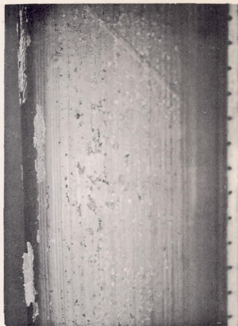
Lower surface after ice removal. Section drag coefficient, 0.0122; lift coefficient, 0.578.
