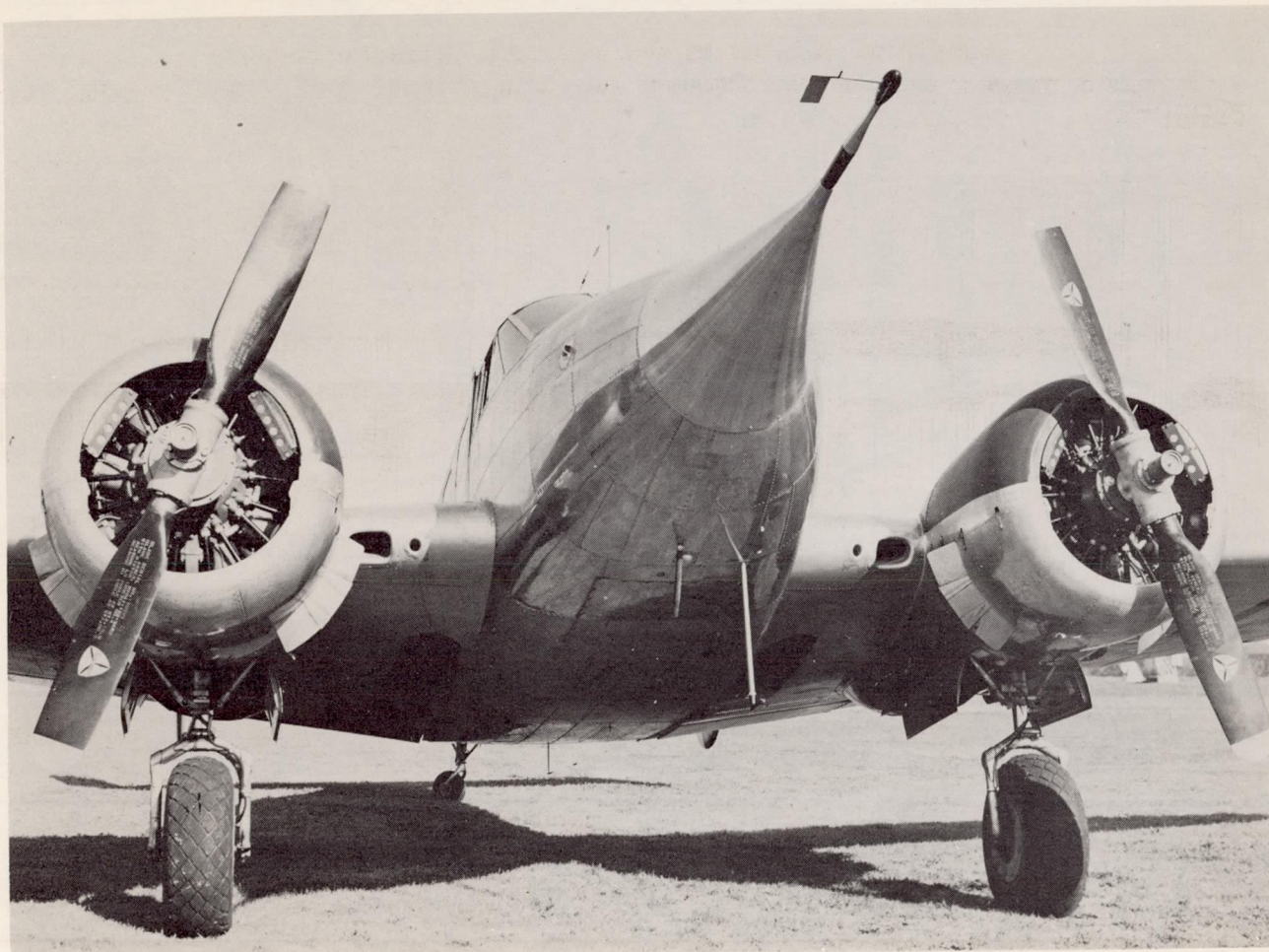
(a) Nose boom and angle-of-attack-vane installation.
