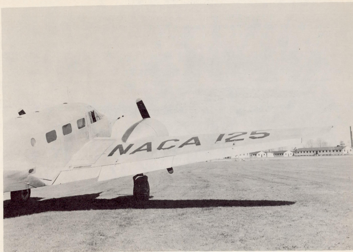
(c) Gust-alleviation flap control in the deflected position. Note that flap and aileron move as one control and that inboard flap is fixed in neutral position. L-88847
