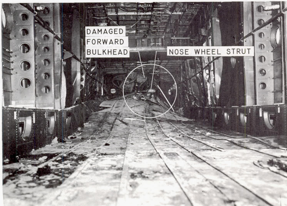
Figure 13. - Nose gear driven into cabin.
