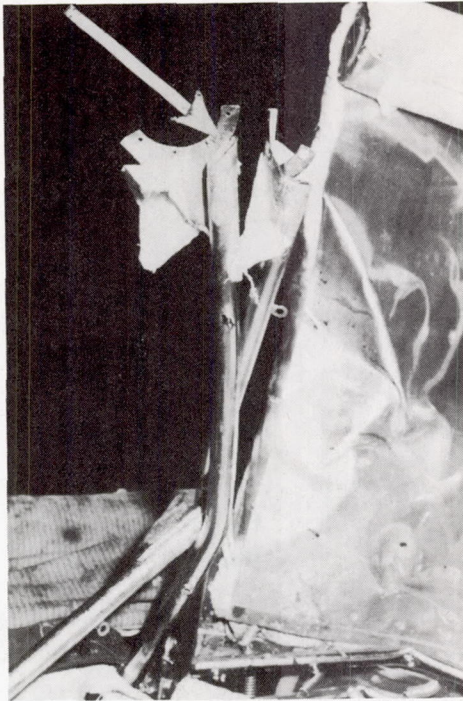
Figure 23. - Spear-like point formed by broken seat back tubing. (Photograph supplied by Aviation Crash Injury group of Cornell University.)
