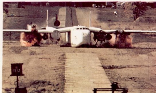
(b) Flames at engine tailpipe, 0.75 second after initial impact.
