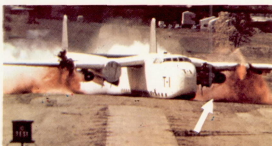
(c) Fuel mist entering left engine, 2.5 seconds after initial impact.
