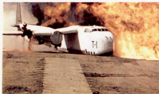
(f) Spread of fire, 4.0 seconds after initial impact.
