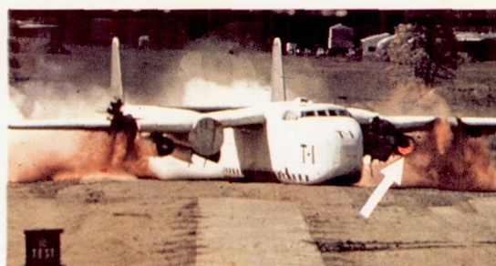
(d) Fire at engine inlet and tailpipe of left engine, 2.6 seconds after initial impact.
