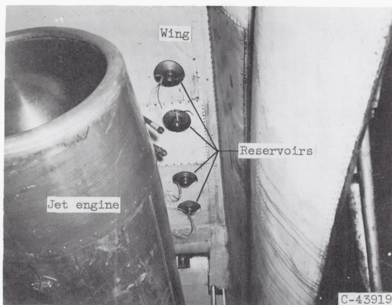
(a) Located in wing root of C-82 cargo airplane.
