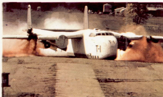
(e) Fire spread to fuel mist issuing from left wing, 2.8 seconds after initial impact.
